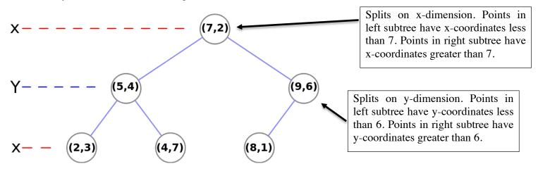
Given an array of Points, we can recursively build up a balanced k-d tree with the following algorithm: At each level of recursion, we will find the median of the Point array based on the dimension index. We will create a new node containing that Point. Afterwards, we will recurse on all the Points before the median point, splitting on the next dimension, setting the results to be the left child. We do the same for the points after the median.
